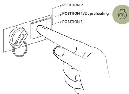
5. Press fully to start the engine (position 2). Once the engine has started, release the button, all lamps go out.
