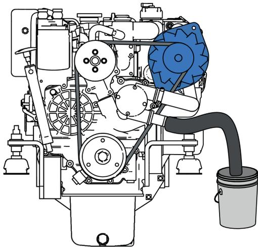
4. Check that no one is in the vicinity of the engine, the propeller and the exhaust outlet. Put the lever in neutral and start the engine.
