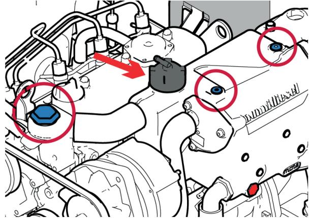
1. Check that the drain plug at bottom of exchanger **(in red)** is properly tightened.
