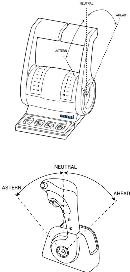
On most boats, the control lever controls both the engine rpm and the gear shift (ahead / astern). However, some boats can be equipped with a separated shift command.
