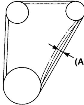
Depress the belt at point (A) and check for a deflection between 7 and 9 mm.
