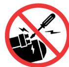
Avoid possible injury or death from engine runaway. Do not start engine by shorting across the starter motor solenoid terminals posts. Engine will start if normal circuitry is bypassed. Start engine from operator's seat.
