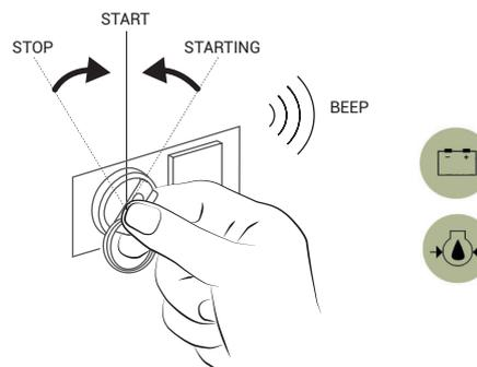
4. Press the Start button halfway (position 1/2) to start preheating. Hold the button for 10 to 20 seconds, depending on ambient temperature to preheat the engine.
