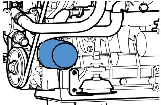
1. Remove the oil filter with a filter wrench tool. Turn the filter counter-clockwise (CCW). Remove the gasket.
