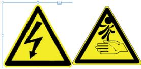
Flammable spray can be generated by heating near pressurized fluid lines, resulting in severe burns to yourself and bystanders. Do not heat by welding, soldering, or using a torch near pressurized fluid lines or other flammable materials.
