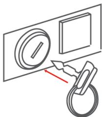
3. Turn the key a quarter-turn to the right (on C4 and A4 panel). All the warning lamps come on and the acoustic alarm sounds. After a few seconds, only the engine oil pressure and Battery charge lamps do lit.
