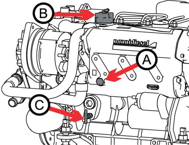
3. Drain off all coolant. Empty the recovery container as well as the hoses used in the process.
