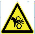
Rotating cooling system fans, belts, pulleys, and drives can cause serious injury. Keep all guards in place at all times during the engine operation. Wear close-fitting clothes.
