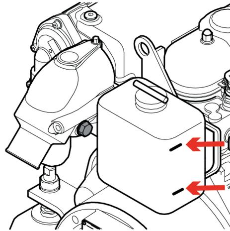
3. Coolant level should stand between the higher and the lower spurs on the side of the tank (red arrows).
